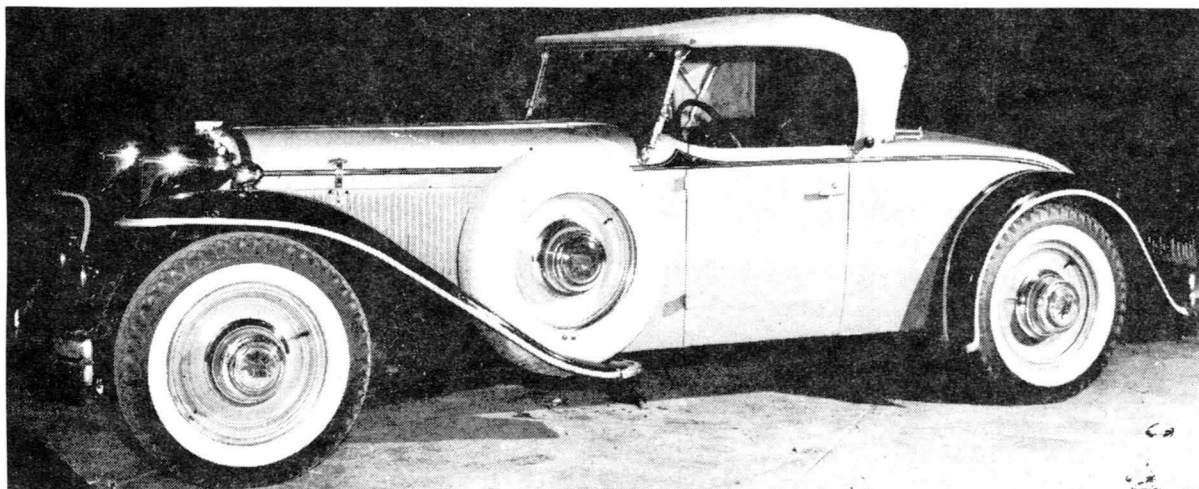
Ruxton roadster, with body by Baker-Raulang, of Cleveland, Ohio. Note the Woodlite “Cat's-Eye” headlights, which were standard equipment on all Ruxton cars except the earliest models.
