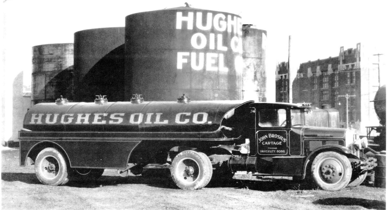
RHYTHM & BLUES? No, Reiland & Bree. This little-known make of truck (or automotive brand, as Elliott would say), sometimes known as R&B, gained some mention and comment in recent issues of SAH Journal. This is a 1931 Reiland & Bree, pulling a 2,600 gallon Heil tank semi-trailer built for the Hughes Oil Company of Evanston, Illinois. Heil factory photo from the collection of James B. Bibb.
