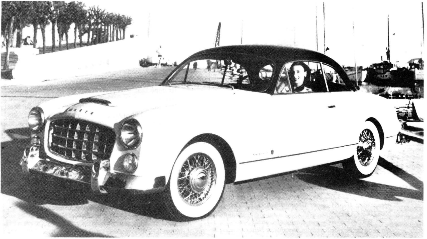
OOH, LA LA! Underneath this lithe French body (by Jean Danino's Facel SA, which would later build the Vega of the same name) lies a flathead Ford V8 engine. The car is, of course, a 1953 Comète sports coupé from Ford of France. From the editor's collection.
