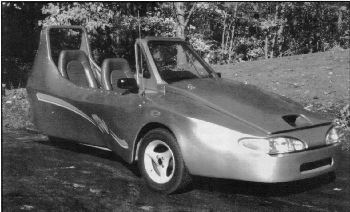
THE WR-70, a one-of-a-kind fiberglass vehicle powered by a Volkswagen diesel engine. Built by Eugene Wright of Pennsylvania, it weighs 1,400 lbs., gets 70 mpg and goes at regular highway speeds. Passengers sit tandem fashion, motorcycle style. It is registered as a motorcycle. Mr. Wright has a patent and is seeking a manufacturer. George W. Green collection
