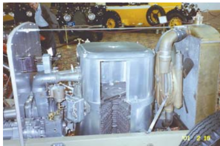
Doble burner and boiler, in the Nethercutt
