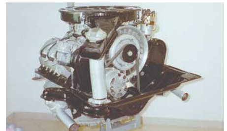
Tatra 613 V6 engine. This engine was simplified compared to the production air-cooled V8 powerplant. This version proposed single overhead camshafts per bank rather than the standard double overhead cams.
