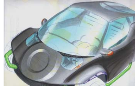
Above: Detail of a larger rendering of the Yamaha design. Artwork is done with markers, chalk and Prismacolor pencil on costly Vincent Vellum. Basic line art was enlarged using a typical office copier.
