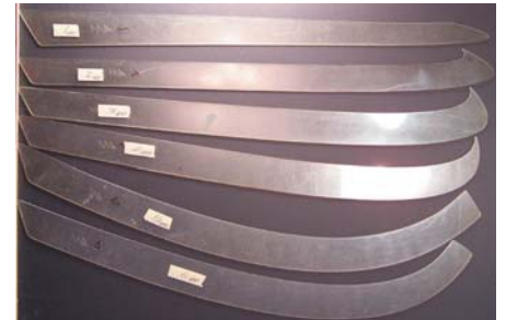
Above: Ship's curves, or “sweeps” which students fabricated in Strother MacMinn's class in 1983.
