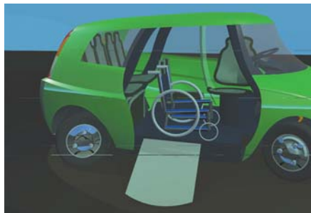
Above and below: 2002 project for a purpose-built taxi. Hand-drawn three-view drawings were scanned to create basis for digital 3D model in the Maya 3D application. Corrupt digital files resulted in strange lines across the images.
