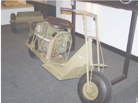
Above: 1944 Cushman Airborne Model 53, M3A4 trailer. Meant to be dropped by parachute with troops. Turf tires, no suspension. Automatic clutch, 40 mph, 100 mile range.
