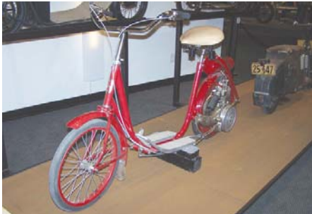
Above: 1920 Briggs & Stratton uses Smith Motor Wheel as integral component. 25 mph, 100 mpg. Sprung seat.
