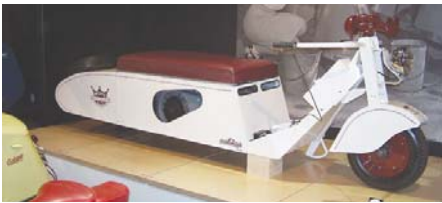
Above: 1947 Mohs King O' The Road. Built by Bruce Baldwin Mohs at age 14. 16hp Onan engine, 60 mph. 13 foot length.
