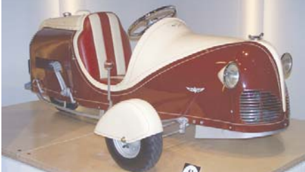
Above: 1939 Moto-Kar Deluxe. 2 hp. Available with cargo body, or pontoons and a propeller for water use.
