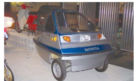
Above: 1984 Zoe Zipper built by Mitsuoka Motors, 50cc Honda engine. Marketed in open and closed versions, single door on the left. 400 pound weight. $3785 in 1984.
