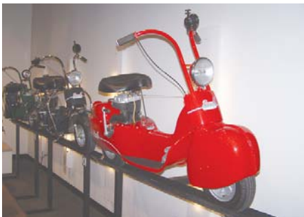
Above: 1947 Powell Challenger C-47. One-cylinder 4-stroke 400cc engine. Los Angeles-based Powell built its own engines, carburetors, ignition and generators.
