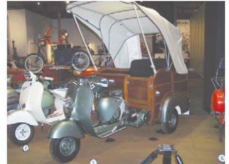
Above: Vespa rickshaw, centrally-mounted engine, independent rear suspension using twin chain cases as trailing arms, one for each wheel.
