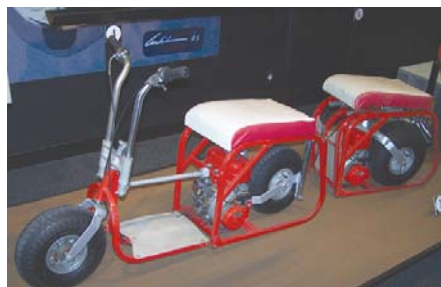
Above: 1960 Fuji Go-Devil folding scooter. 53cc 2-stroke engine, 23 mph. 60 pound weight.
