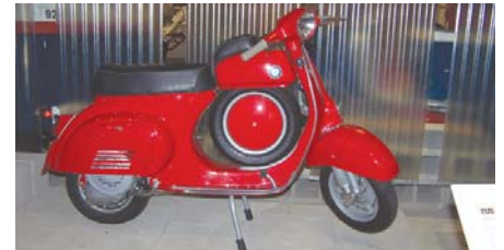
Above: 1966 Vespa Super Sprint 90, lightweight chassis, 90cc engine. Narrow bodywork, centrally mounted spare reduce wind resistance. Tool compartment above spare.
