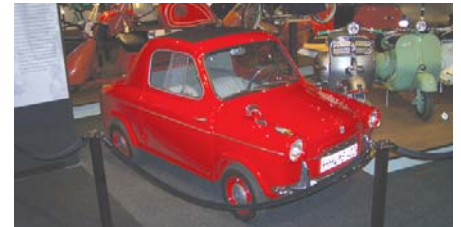
Above: Vespa 400, built in France by Piaggio's subsidiary. Two-cylinder, 2-stroke engine, fan-cooled with a hand-cranked mixer for gasoline and two-stroke oil. Battery in a sliding tray behind the front fascia panel.
