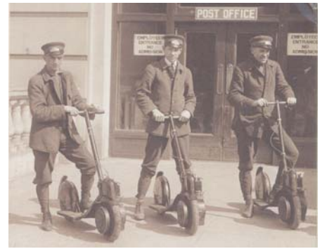
Above, Below: Autoped scooters built from 1915-1921 in New York. The 155cc front-drive stand-up scooter was controlled by pushing forward or back on the steering column. Idea resembles an in-line Segway, 95 years ago.
