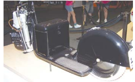
Below: 1917 Kenilworth by Booth Brothers in the UK. One cylinder, 4-stroke engine. Kerosene headlamp, bicycle brakes, sprung seat.
