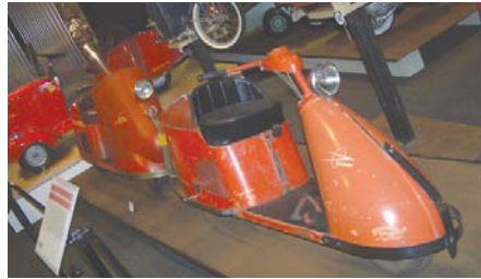
Above: 1946, 1948 Salsbury Model 85 scooters. 6hp, 4-stroke engine, 45 mph, 65 mpg. Built in Pomona, California, automatic shifting, pedals for brake and accelerator. Sole surviving Deluxe model features a front fairing.
