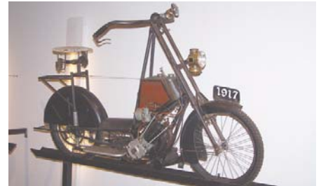
Below: 1917 Kenilworth by Booth Brothers in the UK. One cylinder, 4-stroke engine. Kerosene headlamp, bicycle brakes, sprung seat.
