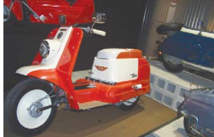
Above: Harley-Davidson Topper H, horizontal single-cylinder engine with CVT belt transmission.
