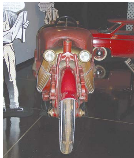
1913 Scripps Booth Bi-Autogo, above and right , pictured at the Petersen Automotive Museum. James Scripps Booth conceived the design at age 20, took four years to build the vehicle at a cost of $25,000. The machine had an under-slung chassis and heavy steering due to excess caster angle with wheel-type steering and 3,200 lb weight. Length 184 inches, width 50 inches. Sheet aluminum over wood formed the body, using concealed door hinges. The driver sat in a single central seat, two passenger seats at rear. The main wheels were artillery type, the rear one driven, front steered, with smaller retractable outrigger wheels, in two pairs, for a total of six tires on the ground. The engine was an L-head 90 degree V8, 332 cid, 5.44 liters, 54 hp, with two pistons on each articulated connecting rod assembly. Other novelties were the compressed air starter, aluminum crankcase and gearbox casing, copper tube radiator draped over each side of the vehicle and enclosed chain drive to the rear wheel.
