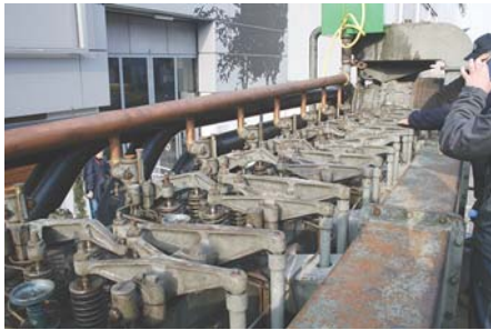
Duvant engine open valve train, above. Bugatti from the Musée National de l'Automobile above right. 1937 Georges Irat MDU with a Ruby engine in as-found condition, right. All photos this page from Lincoln Sarmanian.
