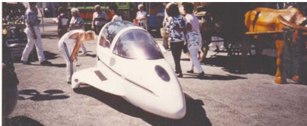
The Autocycle, above , pictured at Expo '86 in Vancouver, BC, Canada, was a Jim Bede design offered by Tomorrow Corporation, Chesterfield, Missouri, starting 1982. The vehicle featured tandem seats, fiberglass body, steel tube frame, driven rear wheel, steered front, the outrigger wheels at center were flexibly mounted, it was legally a three-wheel motorcycle. The factory was listed in Fairhope, Alabama in publicity and plans for home-building the car were available. The Autocycle weighed 575 lbs, powered by a Honda 250cc two-cylinder with a five-speed gearbox for $3995. Optional powertrain configurations: Kawasaki 305cc two-cylinder, belt drive, $4655; Honda 450cc two-cylinder automatic, $5545; Honda 750cc four-cylinder 5-speed, $7195. Litestar 700, above right , weighed 820 lbs, was 194 inches long, 76 inches wide, 54 inches high, claimed drag coefficient of .092. A liquid-cooled shaft-drive motorcycle powerplant was listed, with a warrantee of up to 5 years, 50,000 miles. Distributed by Earthship Enterprises in San Diego, California, among others, with plants in Scranton, Iowa, and later Owosso, Michigan. The Pulse GCRV, or Ground Cruising Recreational Vehicle, below , was offered from 1985-1990 by Owosso Motor Car Co, Owosso, Michigan. Empty weight had increased to 1050 lbs.
