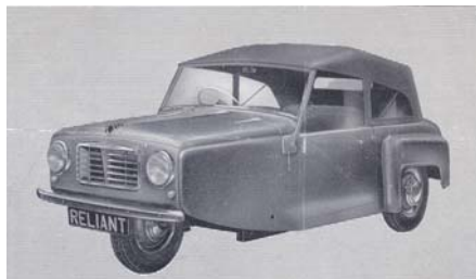
Reliant Regal "Mark I," above, with composite hardwood and metal panel bodywork. Three wheel hydraulic brakes.
