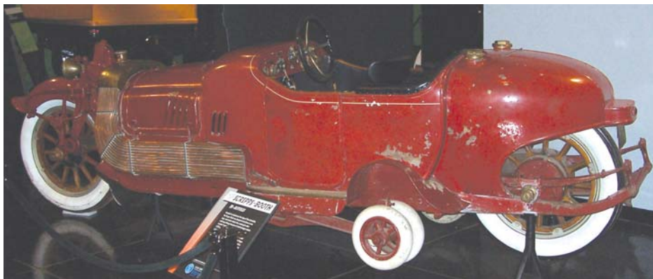
1913 Scripps Booth Bi-Autogo, above and right , pictured at the Petersen Automotive Museum. James Scripps Booth conceived the design at age 20, took four years to build the vehicle at a cost of $25,000. The machine had an under-slung chassis and heavy steering due to excess caster angle with wheel-type steering and 3,200 lb weight. Length 184 inches, width 50 inches. Sheet aluminum over wood formed the body, using concealed door hinges. The driver sat in a single central seat, two passenger seats at rear. The main wheels were artillery type, the rear one driven, front steered, with smaller retractable outrigger wheels, in two pairs, for a total of six tires on the ground. The engine was an L-head 90 degree V8, 332 cid, 5.44 liters, 54 hp, with two pistons on each articulated connecting rod assembly. Other novelties were the compressed air starter, aluminum crankcase and gearbox casing, copper tube radiator draped over each side of the vehicle and enclosed chain drive to the rear wheel.
