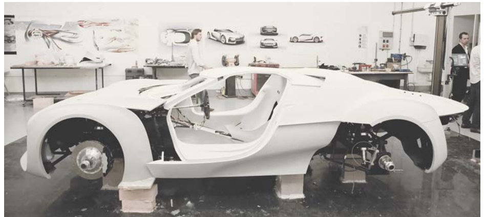
2008 "GTbyCitröen" concept car while under construction. Based on a virtual vehicle from the game Gran Turismo 5 , the car was fitted with a full interior and seats for demonstration purposes. Length: 4960mm (195.2 inches), width 2080mm (81.9 inches) and height of 1090mm (42.9 inches.) Wheels are diamond-effect 21-inch units. Images: Citroën Presse.
