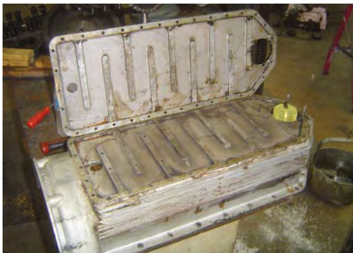
The unique oil cooling and filtration design of the Lancia engine.
