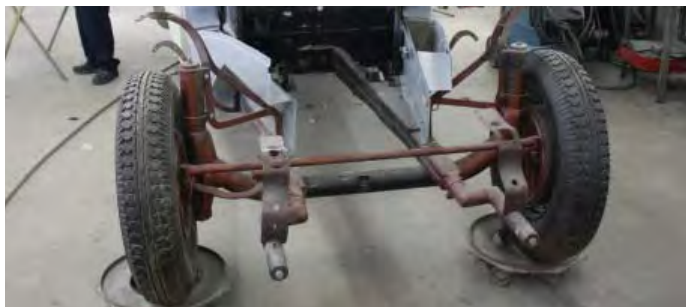
Restoration: a view of the exposed sliding pillar front suspension.
