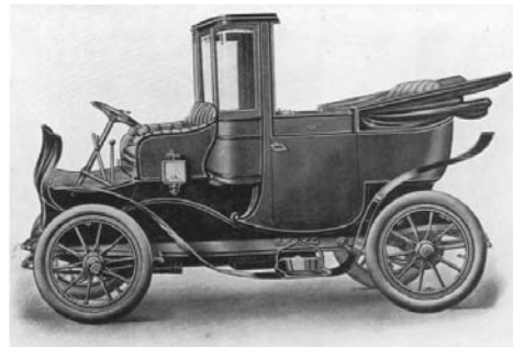
Above: the Rolls-Royce Landaulet Par Excellence as it appeared in the company's 1906 catalogue. The chassis was almost identical to the Legalimit; the main difference was the position of the steering wheel.
