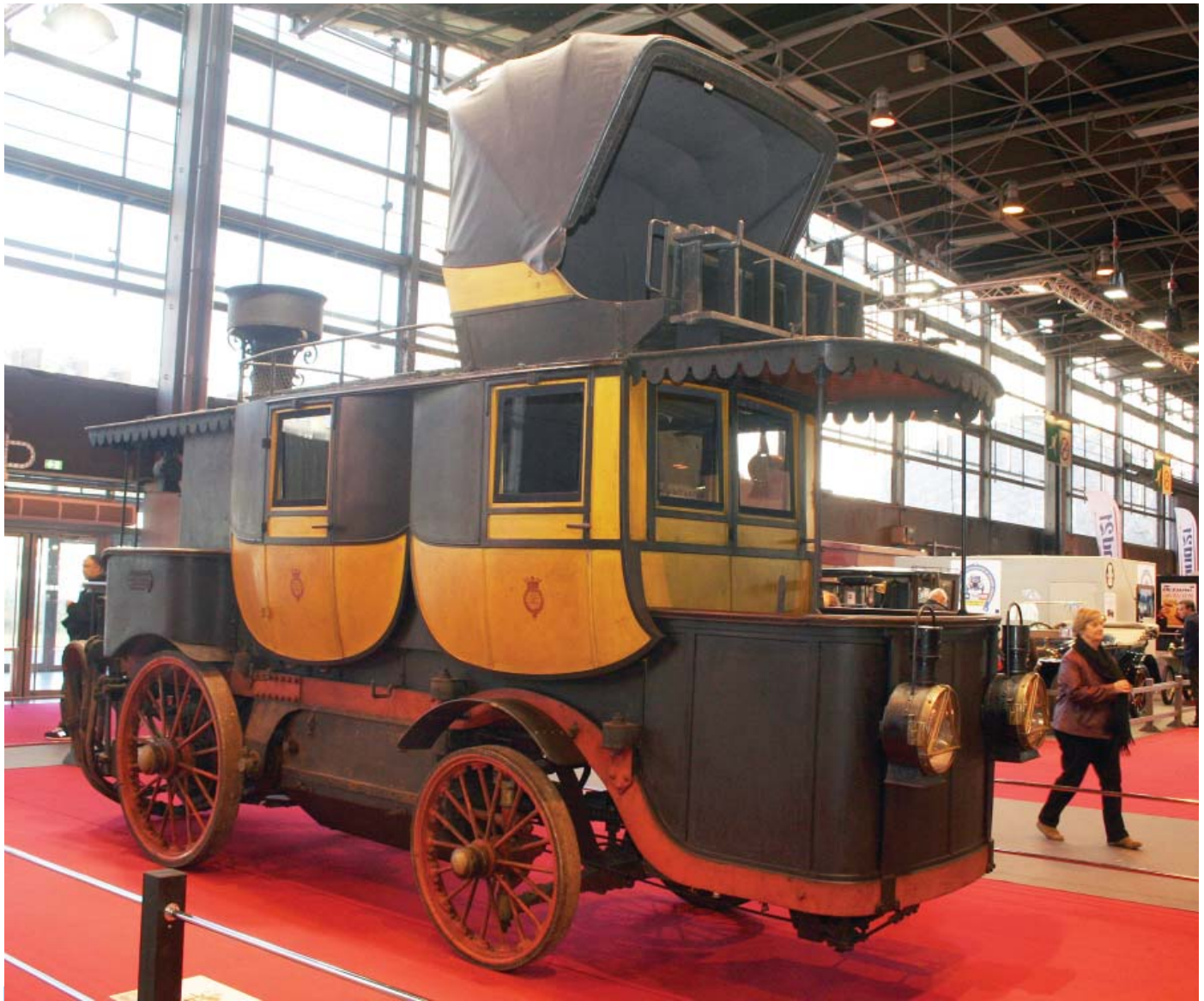
Luxury car, 1885: The diligence à vapeur built by Amédée Bollée Père for the Marquis de Broc can carry 16 passengers at 10 mph.
