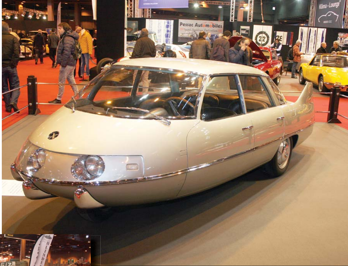
Above: Shades of the Gordon Diamond: The 1960 Pininfarina PFX has four wheels in a diamond pattern, is powered by a 1,889 cc. four-cylinder engine. Left: How to streamline a 2CV: Philippe Charbonneaux's lines smooth out Citroën's basic car, but there's not much one can do with the "greenhouse." Below: French Curves: Cabriolet body by Carrossier Pourtout looks at home on Spirit of Motion Graham.
