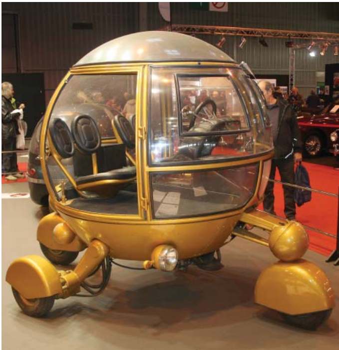
Created in 1970, the spherical l'Automodule is powered by a 248 cc. two-stroke engine and has a hydraulic suspension that makes it dance.
