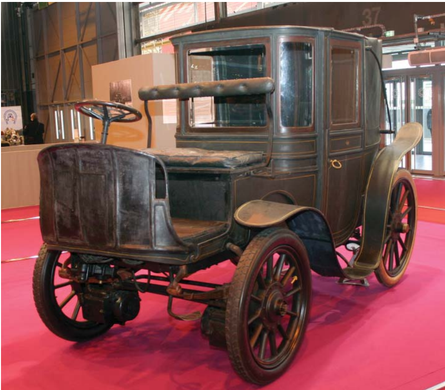
1906 Krieger Landauet Electricque has an electric motor on each front wheel.
