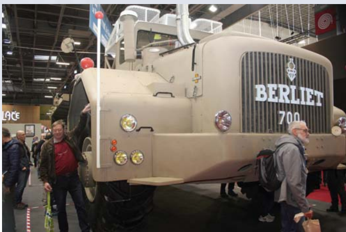
Liliputian show-goers emphasize the enormity of this 700 hp Berliet T100, built for service in Algerian oil fields.
