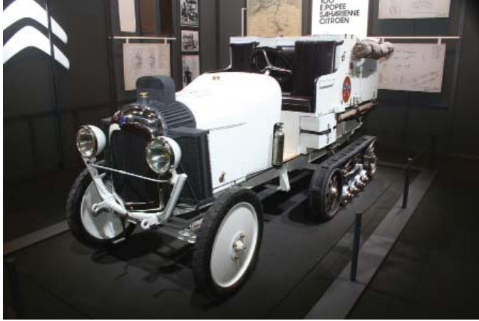
The Citroën display highlighted the tracked “Kegresse” models built in the 1930s for use in the desert.
