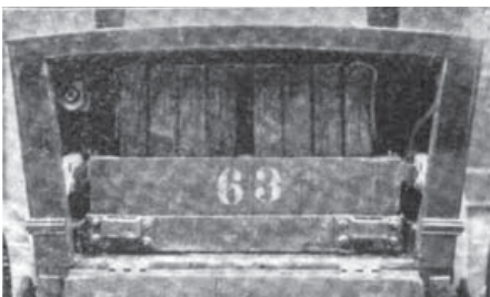
Above and below: before and after a box sleeve with its batteries is placed in a cab as shown at the bottom of page 9. Right: a spent set of batteries is charged while in its sleeve.
