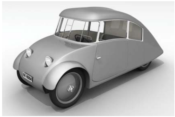
3D model created from an original design drawing by Josef Ganz for a 4-seater, rear-engined “volkswagen” with Paul Jaray-inspired streamlined bodywork, 1933.
