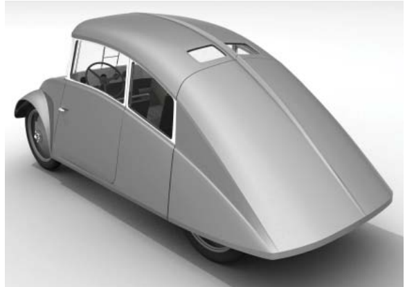
The rear-mounted engine sits behind a huge engine lid that also covers the rear wheels.
