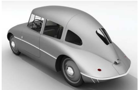
The typical teardrop-shaped back of the Jaray-Ganz “volkswagen.”
