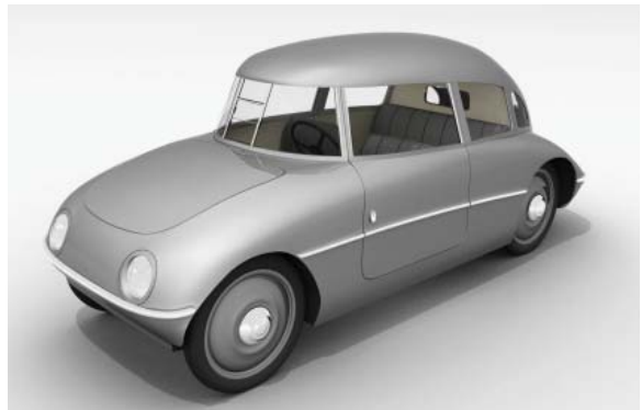
3D model created from an original blueprint by Paul Jaray for a streamlined, 4-seater “volkswagen” on the Ganz-designed chassis of the Bungartz Butz, 1934.
