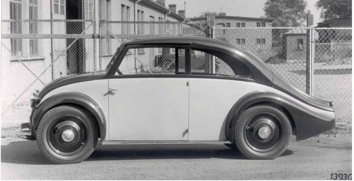
The 1931 Mercedes-Benz 120 prototype featured a rear-mounted, air-cooled 4-cylinder engine and swinging rear half-axes.
