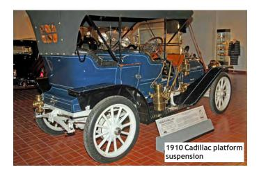
the front and rear axles until superseded by independent systems and coils. The 1962 Chevy II introduced a single leaf for each rear spring.
