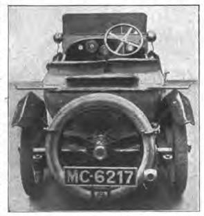
Rearward view of the 12 h.p. 1920 Bugatti, showing the attachment of the reversed quarter-elliptic springs to the tubular rear cross-member
