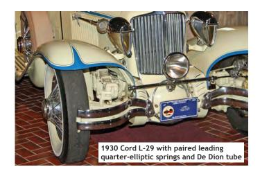
In the former, quarter-elliptic springs were used all around, with the front springs leading, or pointing diagonally forward, and the rear springs trailing. The Chevrolet 490 was designed by Alfred Sturt. Interestingly, a period brochure refers to the rear springs as cantilever, but in reality, they are quarter elliptical. In theory, this arrangement would have offered anti-dive braking properties but in reality, front brakes were not offered on the front axle.
