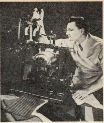
This testing machine finds out how well automobile seat cushion upholstering will wear against the material from which suits and overcoats are made. Strips of the upholstery are rubbed against the suit material until the wearing qualities have been determined.
