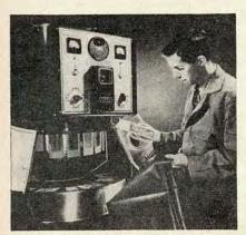
This fadeometer tests the resistance of fabric and leather colors to sunlight and moisture. After getting a dose of sunlight and moisture equal to several years of normal exposure, the fabric is taken from the testing machine and compared with its original colors.
